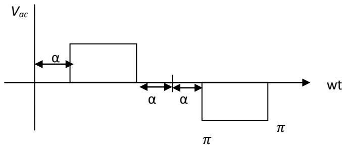
**Fig 1:** Inverter output for amplitude and harmonic control
